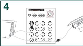
Connect all lamps to their respective ballast, then connect the ballasts to the LMU. Refer to the Lamp Distribution Guide provided with your LMU to prevent Overloading.
