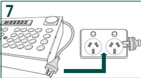
Connect the control cable to the PowerPoint and turn the switch ON.
